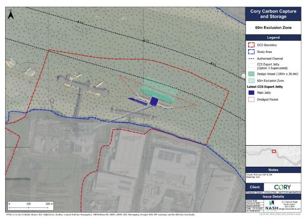
Figure 60: New Proposed Jetty Design Overlaid on Option 3.
