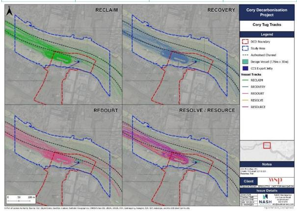
Figure 21: Vessel Tracks, Cory Tugs (PLA AIS 22)
