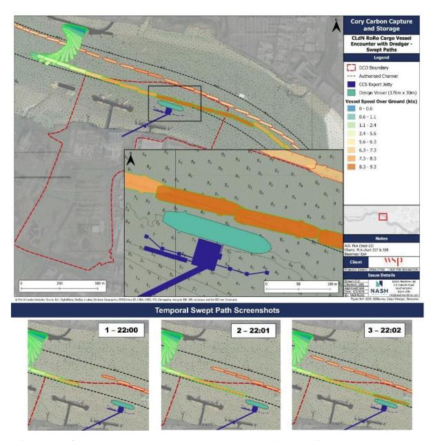
Figure 47: Swept path analysis showing the dredger *Hanson Thames* and the cargo vessel *Wilhelmine* on 30-Oct-23 at approximately 22hr00
