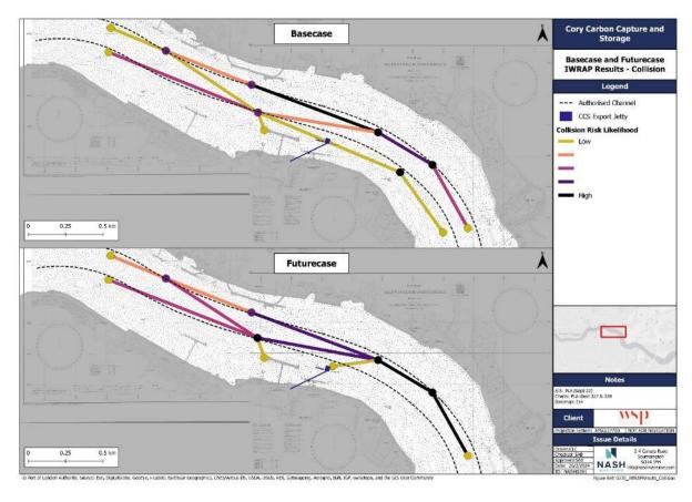
Figure 52: Collision IWRAP Results
