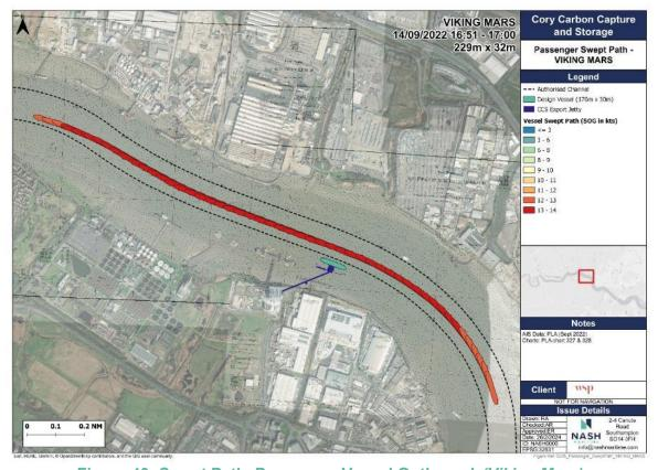
Figure 40: Swept Path, Passenger Vessel Outbound (Viking Mars)
