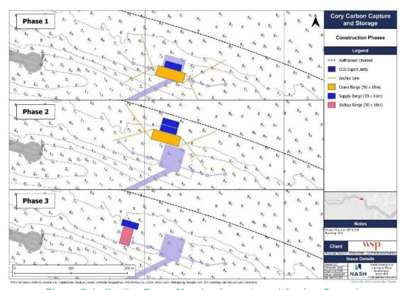
Figure 7: Indicative Barge Mooring Layouts and Anchor Spread.
