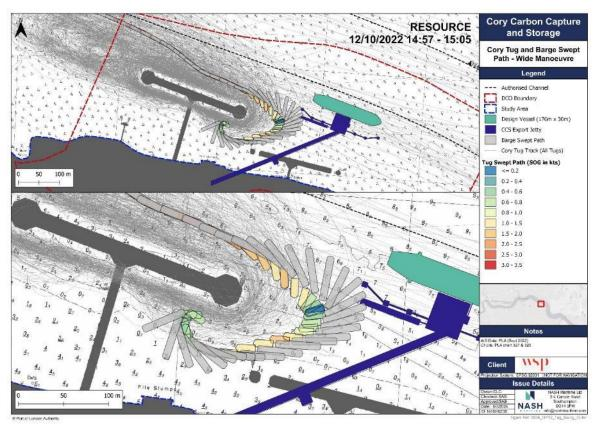
Figure 43: Cory Tug and Barge Flood Tide Berthing
