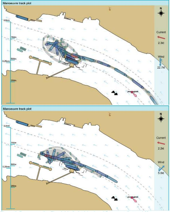
Figure 5: Representative Flood tide Arrival (top) and Departure (bottom) Manoeuvres.
